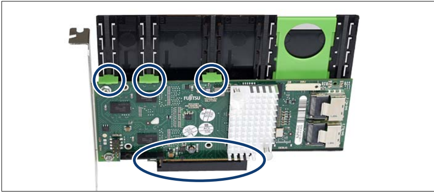
Figure 66: Inserting the expansion card in the removal tool
